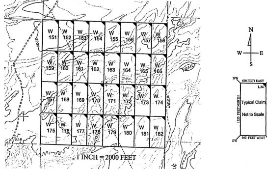
The above map depicts the W- 15.5 placer mining claim, which is located in Section(s) \_\_\_\_\_\_ 24\_\_\_\_, Township \_\_ North, Range \_\_\_13\_\_ West. Gila and Salt River Baseline and Meridian, Mohave County, Arizona. The claim corners and Location monuments are marked by 2 inch by 5 foot wooden post with aluminum tags. The bearings and distances between claims are depicted on the map.
