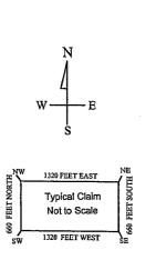
\_\_\_ placer mining claim, which is located in Section(s) 12 , Township The above map depicts the W - 1/North, Range 13 West. Gila and Salt River Baseline and Meridian, Mohave County, Arizona. The claim corners and Location monuments are marked by 2 inch by 2 inch by 5 foot wooden post with aluminum tags. The bearings and distances between claims are depicted on the map.
