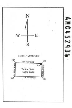
The above map depicts the W-12placer mining claim, which is located in Section(s) 12. Township North, Range 13 West. Gila and Salt River Baseline and Meridian, Mohave County, Arizona. The claim corners and Location monuments are marked by 2 inch by 5 foot wooden post with aluminum tags. The bearings and distances between claims are depicted on the map.
