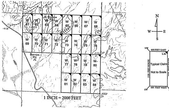
The above map depicts the  $\underline{W}$  -  $\underline{G}$  2 placer mining claim, which is located in Section(s) \_\_\_\_\_36\_\_\_, Township North, Range 13 West. Gila and Salt River Baseline and Meridian, Mohave County, Arizona. The claim corners and Location monuments are marked by 2 inch by 5 foot wooden post with aluminum tags. The bearings and distances between claims are depicted on the map.
