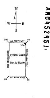
The above map depicts the w = 2.7placer mining claim, which is located in Section(s) 6. Township North, Range 12 West. Gila and Salt River Baseline and Meridian, Mohave County, Arizona. The claim corners and Location monuments are marked by 2 inch by 2 inch by 5 foot wooden post with aluminum tags. The bearings and distances between claims are depicted on the map.
