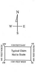
The above map depicts the W - 7 placer mining claim, which is located in Section(s) 12 , Township 15 North, Range 13 West. Gila and Salt River Baseline and Meridian, Mohave County, Arizona. The claim corners and Location monuments are marked by 2 inch by 2 inch by 5 foot wooden post with aluminum tags. The bearings and distances between claims are depicted on the map.
