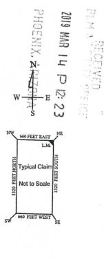
The above map depicts the <u>W-33</u> placer mining claim, which is located in Section(s) <u>6</u>, Township The claim corners and Location monuments are marked by 2 inch by 2 inch by 5 foot wooden post with aluminum tags. The bearings and distances between claims are depicted on the map.
